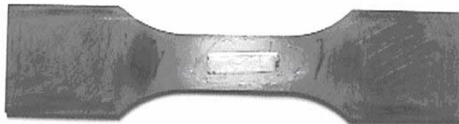
Fig. 1. The shape of sample and typical orientation of the «smart» sensor.
