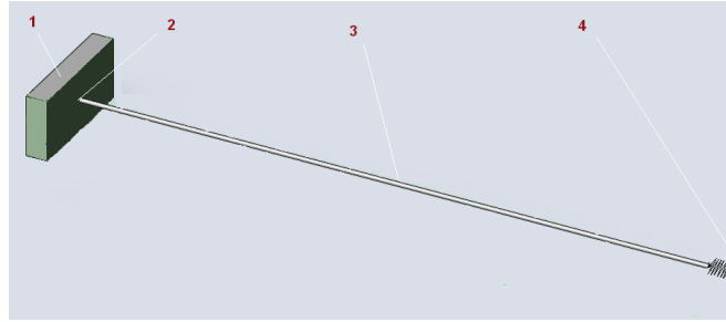
Figure 1. Configuration of an anchor against landslide construction: 1 - a retaining wall; 2 – a tightener; 3 - a rod and 4 - a locking device
