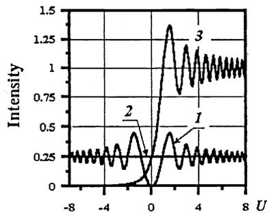
Figure 6 [10]. Khizhnyak's decomposition of the diffraction field behind a half-infinite opaque screen: 1 - the ED(*dislocation*)W, 2 - the plane wave, 3 - the resulting diffraction wave.
