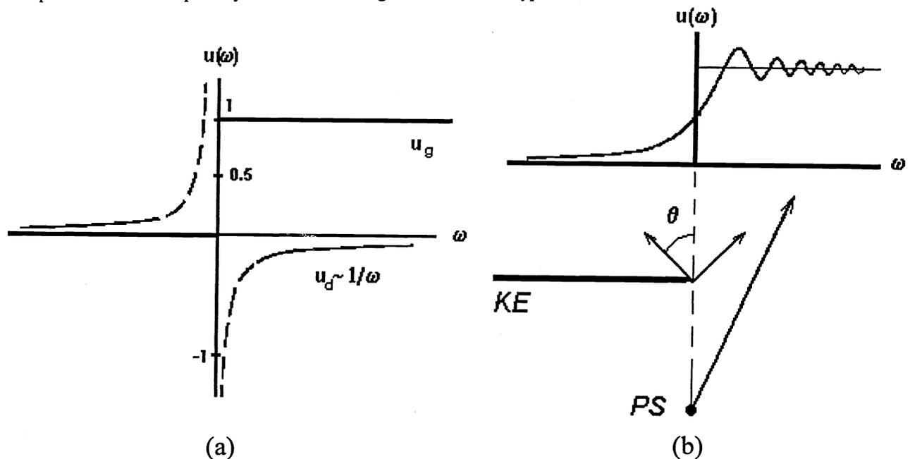
Figure 4. Components of a knife-edge diffraction field following to the Rubinowicz representation of the Kirrhoff's diffraction integral (a):  $u_g$  is the GOW,  $u_d$  is the EDW, and formation of a knife-edge diffraction pattern (b): PS - primary source, KE - knife edge,  $\theta$  is the diffraction angle.
