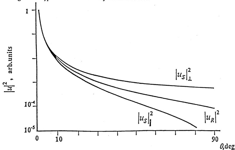
Figure 2. Behavior of diffraction field at large diffraction angles predicted by the rigorous (vector) Sommerfeld's solution of diffraction problem,  $|u_S|^2_{\perp}$  and  $|u_S|^2_{\parallel}$ , and by scalar diffraction theory,  $|u_R|^2$ .
