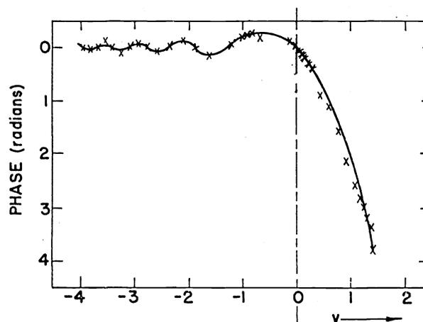
Figure 8 [<sup>8</sup>]. Phase in the knife-edge diffraction pattern calculated using Fresnel integral and the Cornu's spiral (a curve) and determined interferometrically (crosses).
