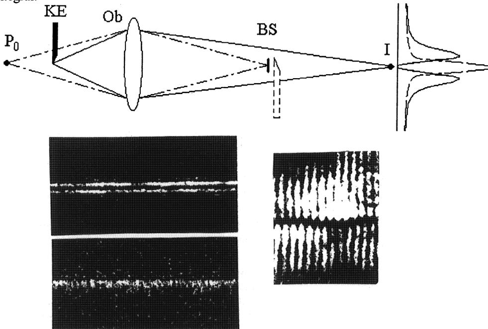
Figure 5. Sketch of dark-field observation experiments following by Toepler and Foucault:  $P_0$  - primary source, *KE* - knife edge, *Ob* - objective, *BS* - blocking screen, *I* - image; double-contour image (following Toepler), single-contour image (following Foucault), and interference testing of a phase structure of the doubly contoured dark-field image.
