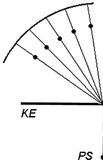
Figure 3. Sketch of the Kalashnikov experiment: *PS* - primary quasi-point source, *KE* - knife-edge; black circles are the pins followed by a photographic film.
