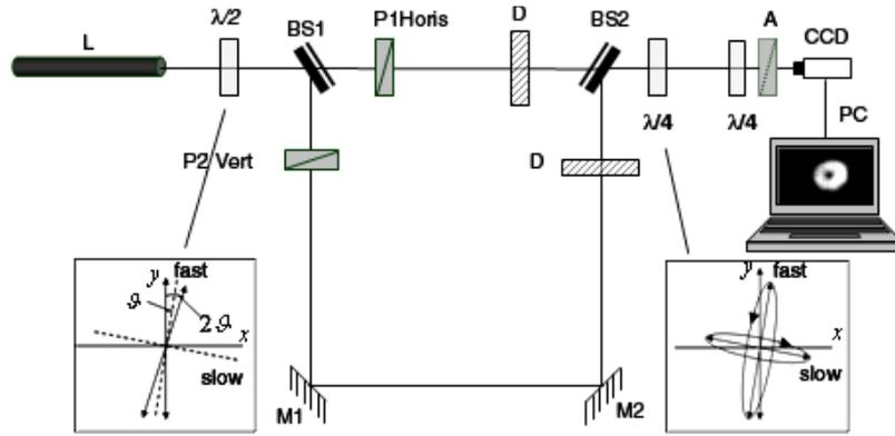
**Figure 4.** Experimental arrangement: L—laser;  $\lambda/2$  and  $\lambda/4$ —half-wave and quarter-wave plates, respectively; BS1, BS2—beamsplitters; P1, P2—polarizers; M1, M2—mirrors; D—diffusers; A—linear analyzer; CCD—CCD camera; PC—personal computer. Action of a half-wave plate and a quarter-wave plate at the input and output of the interferometer, respectively, is shown in insets.
